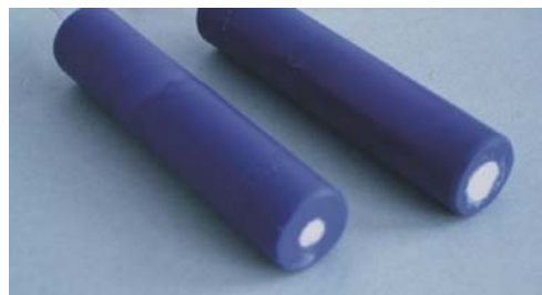
Fig. 4 Photo of all-solid reference electrodes according to Fig. 2c with different sizes of the free surface of the diaphragm
